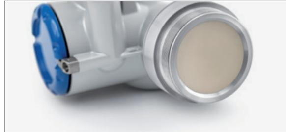
This type of antenna is available for the 80 GHz frequency range radar systems. Here, a dielectric lens is given at the interface between the radar and the tank or silo and can directly fulfill the function of a 'barrier element'. Advantageously with this design, the overall length of the antenna is very small, while offering a good electrical matching.
